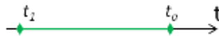
Figure 10: Activation domain of the Simple direct STSD: for sequences characterized by interspike intervals comprised between 0 and a certain value t_a , the detection is positive; otherwise the detection is negative.
