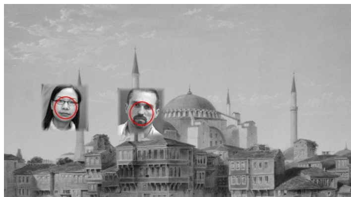
Figure 22: Test Image with face detection applied on by a trained classifier with optimal parametric values
